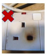
Take a few minutes to make sure you are not overloading sockets, that you are using extension leads correctly, they do not present a trip hazard, and that charging devices are placed on hard, non-flammable surfaces. We all need to keep electrically safe whilst working from home.
