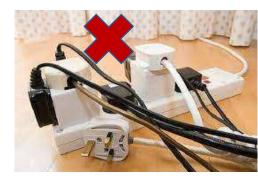
the devices does not exceed the lead's wattage rating. If it did, it could lead to the plug in the wall overheating, causing a fire. The maximum rating of any extension lead for normal domestic use is 13 amps, but some are rated at only 10 amps or less. The rating should be clearly marked on the underside of the extension lead. Extension leads should meet the requirements of BS5733 and parts of BS1362-2.
