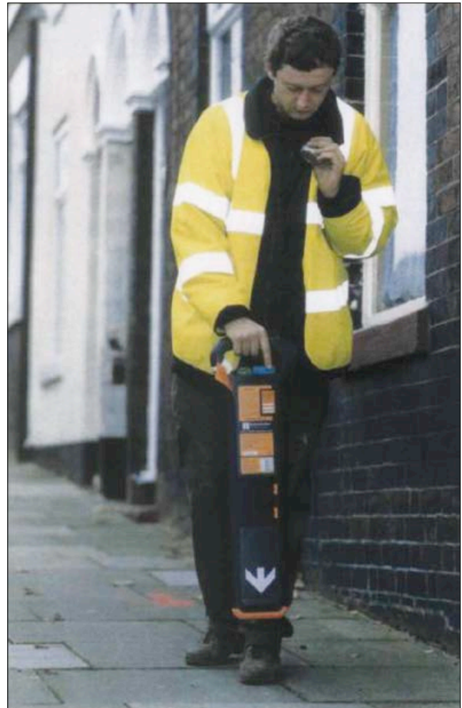
Figure 5 Using a cable locator
